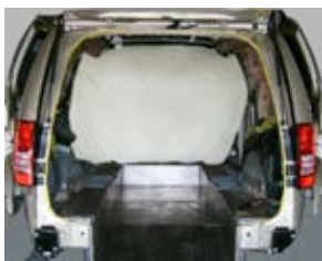
Steel pan welded on the frame and fully sealed
