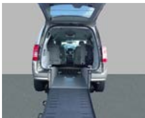
Completed conversion with light-weight aluminum ramp system
